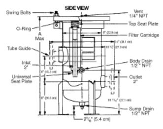
Data presented in this section represents typical dimensions for MSO housings. For critical requirements, request a certified drawing.
