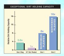
These two graphs compare high efficiency bags and 10" standard pleated filter cartridges with Marksman POLY-FINE® II elements. Comparison is typical for most grades of filter.
