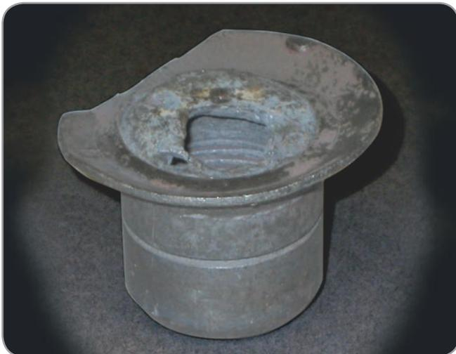
*Damaged NOx burner tip due to contaminants*
