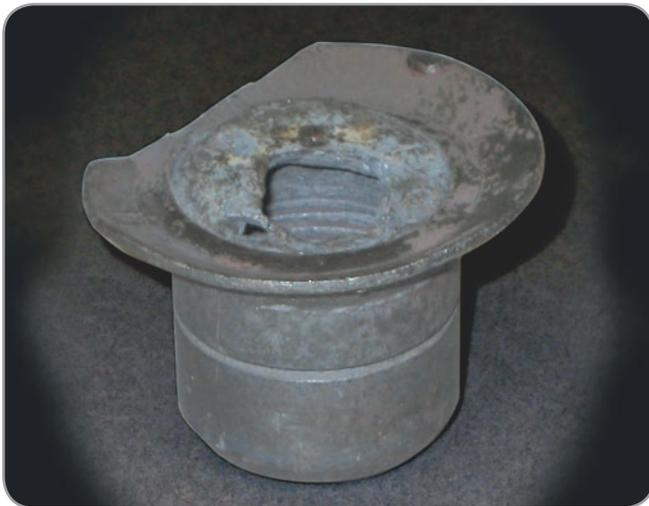
*Damaged NOx burner tip due to contaminants*
