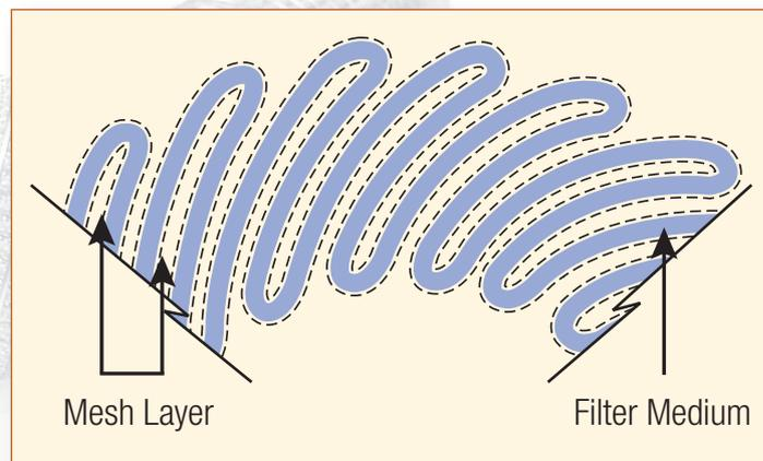
Figure 2: Ultipeat filter element construction
