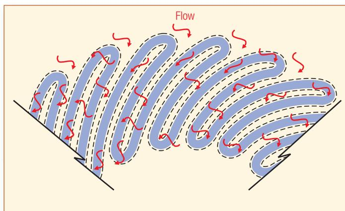
Figure 1: Uniform flow distribution of an Ultipeat filter
