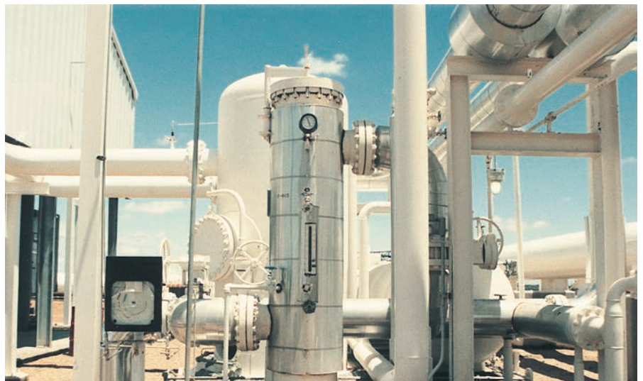
Pall's liquid/gas coalescers remove liquids and solids from hydrogen and fuel gas, protecting turbo machinery and combustion equipment.
