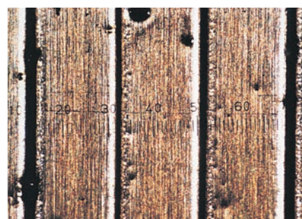
Typical wedgewire element — approximate void volume = 4%.
