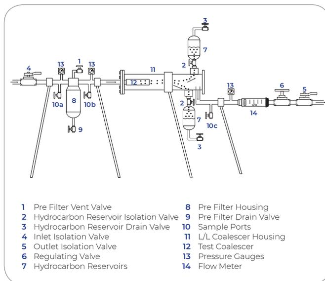
Figure 6: Illustration of Pall pilot scale liquid/liquid coalescer test stand
