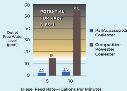
**Figure 3: Effluent Quality – Pall vs. Competition 0.1% Water Ingression, 33 dynes/cm, Vertical Configuration**
