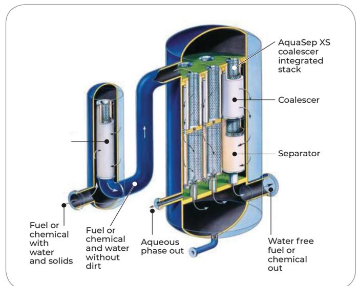
*Figure 5: AquaSep XS Liquid/Liquid Separation System with an Integrated Coalescer/Separator Stack in a Vertical Housing with a Prefilter*
