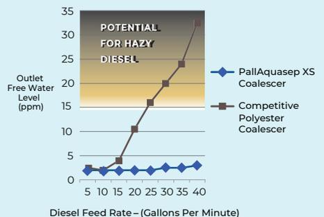
NOTE: Comparison tests were performed in a Pall laboratory with a limited number of 20 inch elements that were purchased through standard commercial channels. Lab results may not be identical to test results with actual process fluid under field conditions.
