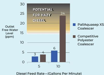
**Figure 2: Effluent Quality – Pall vs. Competition 5% Water Ingression, 33 dynes/cm, Vertical Configuration**
