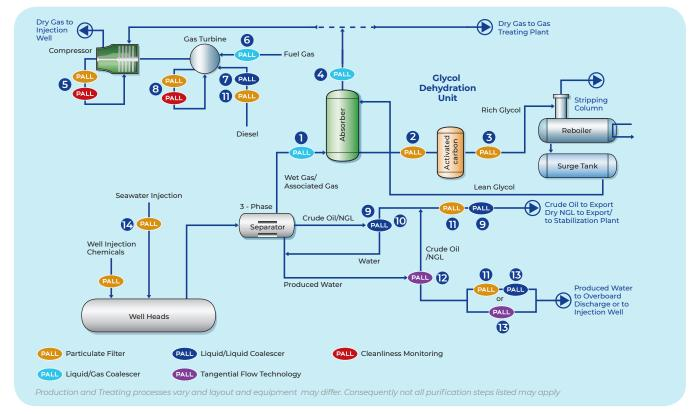
Pall Filtration and Separation Applications at Oil and Gas Production Plants
