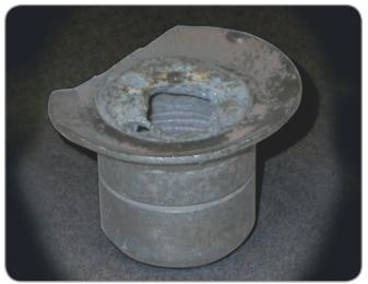
Damaged NOx burner tip due to contaminants
