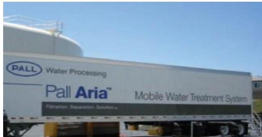
Mobile Water treatment units (MF & RO)
