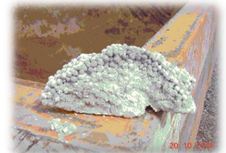
Degraded adsorbent beads - Photo courtesy of CECA
