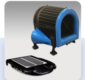
**Aerospace Engine Air Inlet Filters** help address the main reasons for premature helicopter engine failure by minimizing the impact of engine erosion, corrosion and FOD (Foreign Object Damage).
