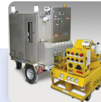
**Commercial and Military Mobile Hydraulic Fluid Purifiers** are a breakthrough in preventive maintenance, saving operators money and time by ensuring operation of aircraft without downtime caused by fluid contamination.
