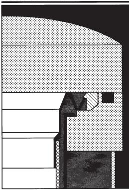
Hermetic seal of filter bag within housing to prevent liquid bypass.
