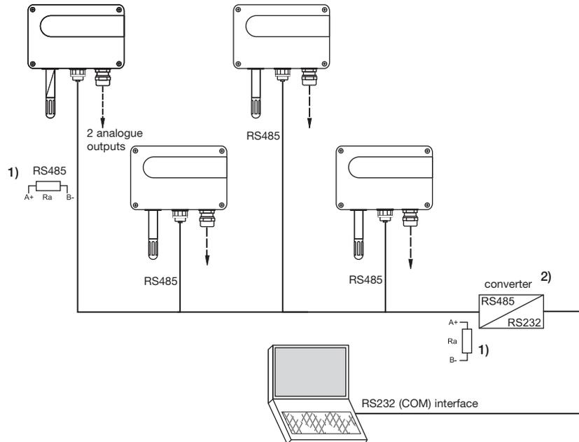
1) Note: to enable optimum expansion, both ends of the network must be terminated with a 100 Ohm resistor.
