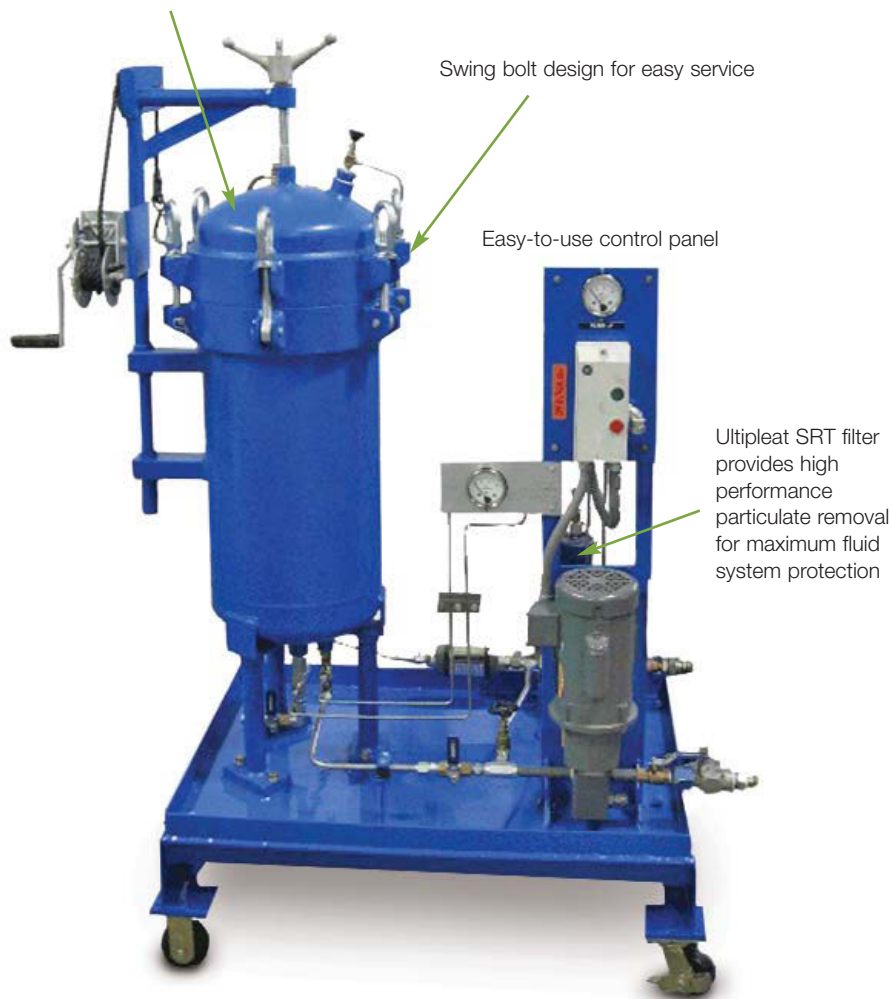
Treatment vessel: Contains three resin bags to capture varnish from mineral oil systems
