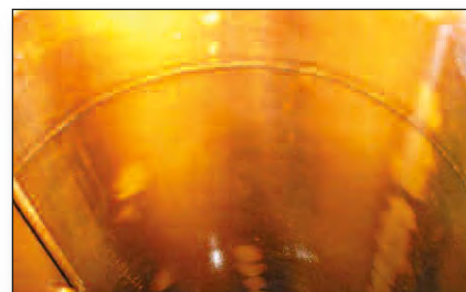
Filter housing internals coated with varnish
