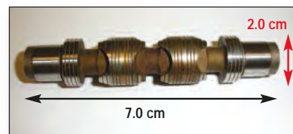
Heavily contaminated servo valve due to varnish deposit
