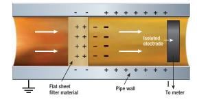
Figure 1. Streaming Current
