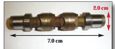
Heavily contaminated servo valve due to varnish deposit
