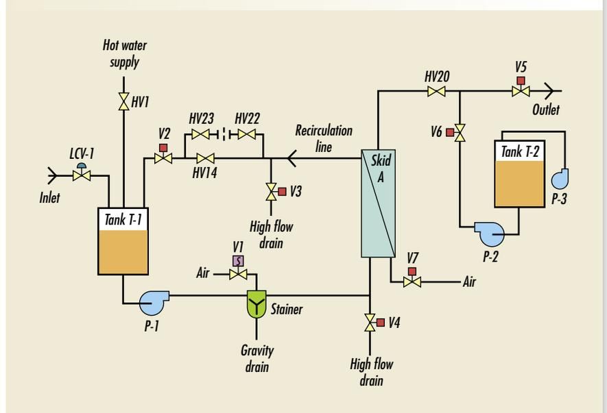
crofiltration for this application would require close monitoring of membrane differential pressure; however, systems utilizing this type of makeup can be set up for enhanced flux maintenance (EFM). A microfilter arranged for EFM uses an additional, small skid that periodically subjects the membranes to short-duration chemical washes to remove accumulated solids, including
