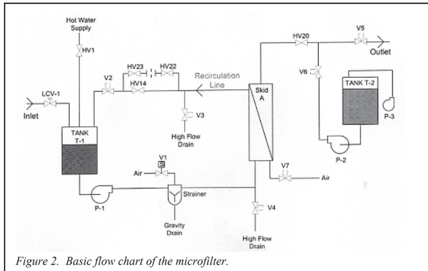
Figure 2. Basic flow chart of the microfilter.
