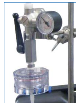
Silt Density Index Test Kit — enables simple water quality monitoring
