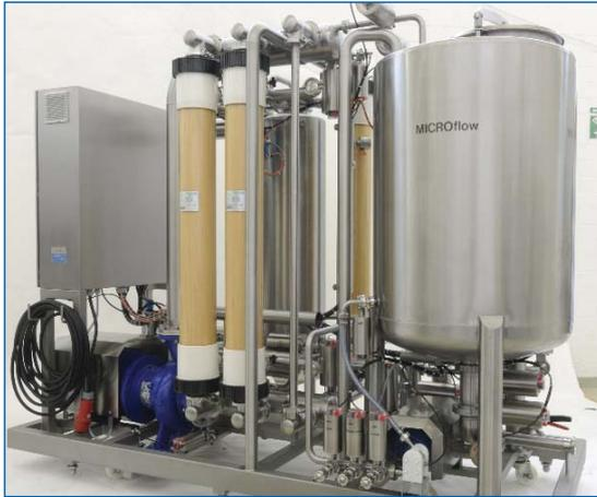
Figure 10d: Membralox Fermenter Broth Clarification System
