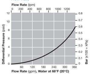
For liquids other than water, multiply differential pressure by fluid viscosity (cP).
