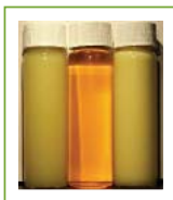
Feed (left), BioDiesel (middle), Coalesced soapy water (right)
