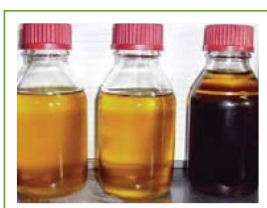
Feed (left), BioDiesel (middle), Coalesced Glycerin (right)
