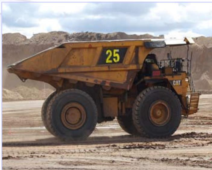
218 Tonne Payload Haul Truck
