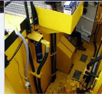
Pall **Ultipleat**<sup>®</sup> SRT filters in diesel fuel applications
