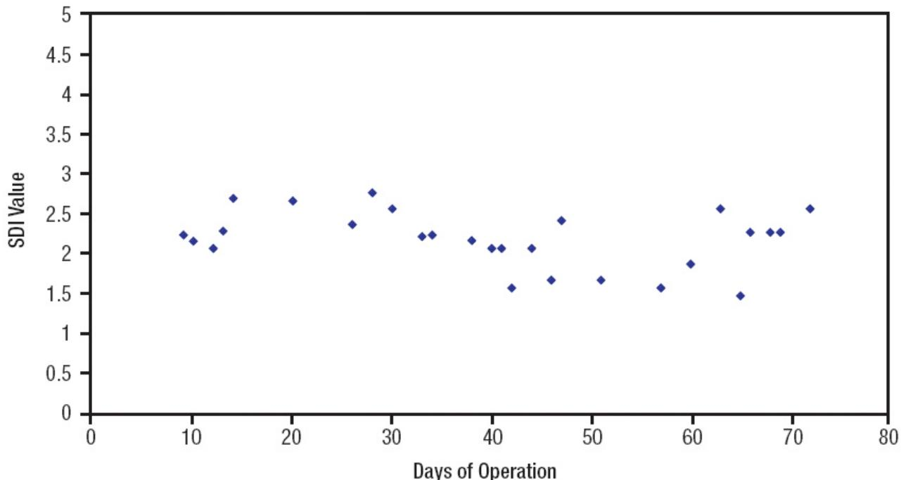
Figure 3: Variation of Silt Density Index after Microfiltration
