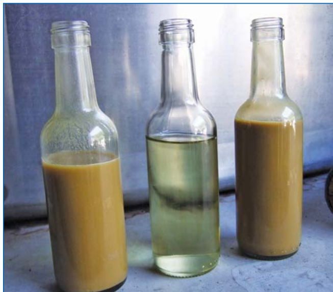
Oenoflow HS must lees samples ( left: feed, middle: filtrate, right: concentrate )
