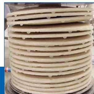
Cell deformities after heat treatment
