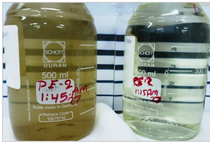
Jet fuel Upstream of filtration Jet fuel Downstream of filtration
