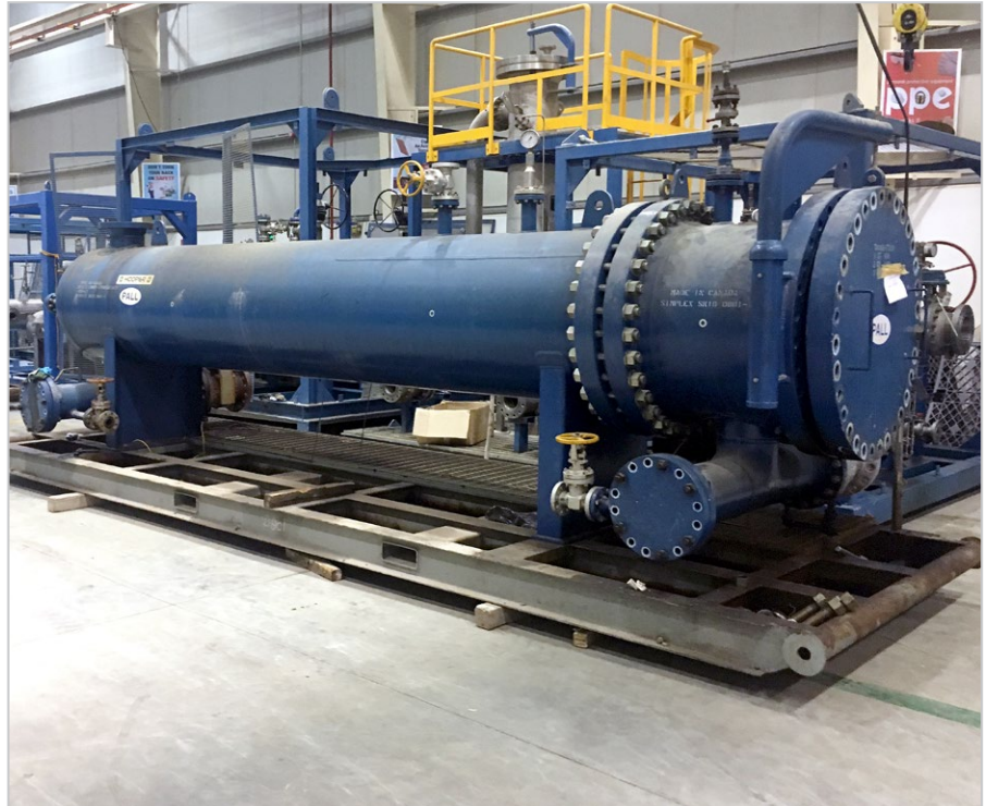
One of two Pall Ultipleat High Flow solid particulate skids
